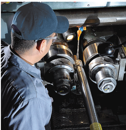
Thread rolling increases strength and eliminates stress risers
